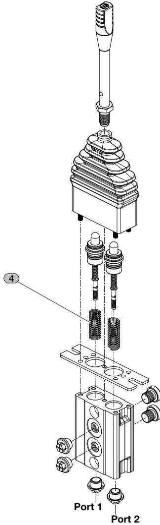
All servocontrols are equipped with 2 return springs (one spring each service port).
