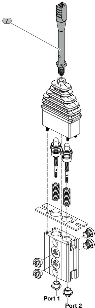
Each rod lever kit includes a rod lever, a nut and a knob. This example shows a rod lever kit EHS1.
