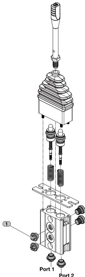
All servocontrols ESJ01A, ESJ01B and ESJ01C include an assembly section kit. Assembly kit for single section is composed by 2 port plugs and 4 plastic plugs. Assembly kits with up to 12 sections also contain tie rods, nuts, growers and o-rings.
