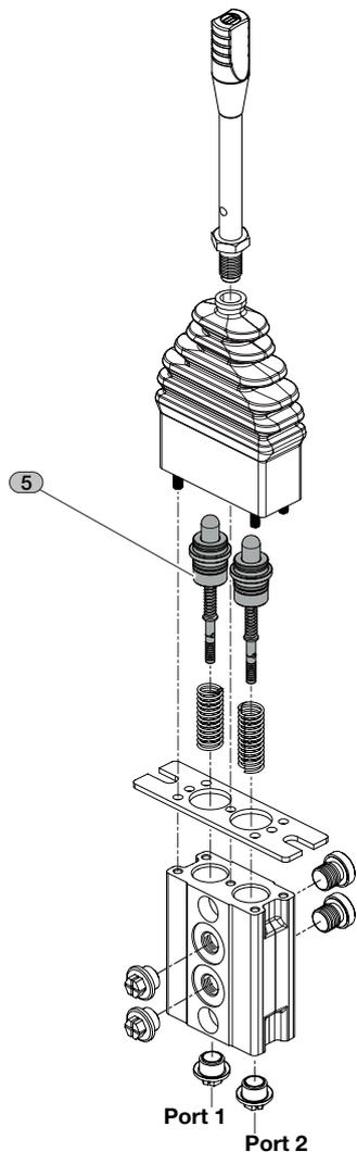
All servocontrols are equipped with 2 metering curves (one metering curve each service port).
