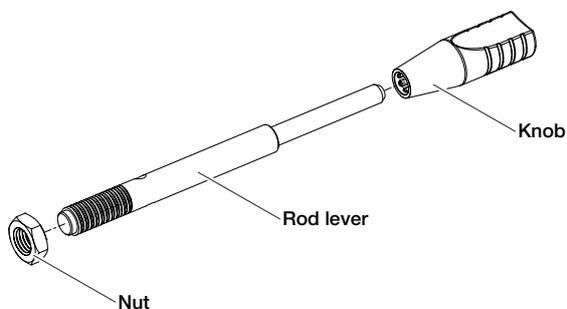
All servocontrols are equipped with a customized control lever.
