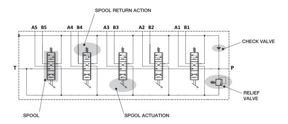
ECM08B/5 with manual actuation in standard configuration.
