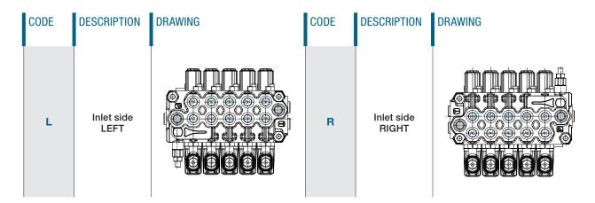
Convention for all ECM08B valves with inlet right (R) or left inlet (L):
