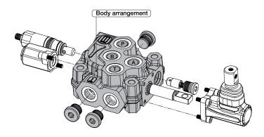
Moboblock control valve body arrangement is available in two configurations: SAE thread or BSP thread. All threads present in each body are equal.
