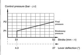
On request are available broken line metering curves with step and broken line metering curves without step. For different values or different applications please contact our Sales Office.
