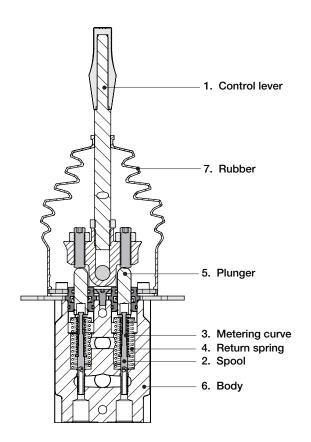
When the control lever is deflected, the plunger is pressed against the return spring and the metering curve. The metering spring initially moves the control spool downwards and closes the connection between the relevant port and tank port T. At the same time, the relevant port is connected to port P via the drilling.
