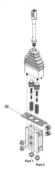
The fixing plate allows the correct installation of the servocontrol on the customer machine system.
