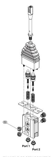
All servocontrols ESJ01A, ESJ01B and ESJ01C include an assembly section kit. Assembly kit for single section is composed by 2 port plugs and 4 plastic plugs. Assembly kits with up to 12 sections also contain tie rods, nuts, growers and o-rings.
