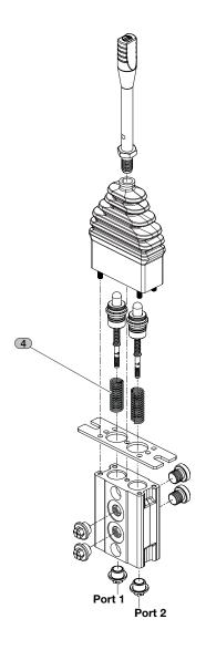
All servocontrols are equipped with 2 return springs (one spring each service port).
