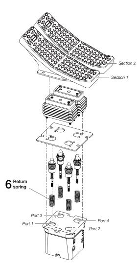
All ESP04A servocontrols are equipped with 4 return springs (one spring each service port).
