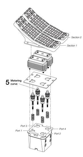
All ESP04A servocontrols are equipped with 4 metering curves (one metering curve each service port).
